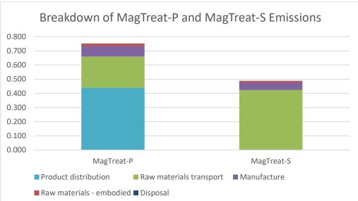
Figure 1: Emissions breakdown of Brucite+'s MagTreat-P and MagTreat-S
